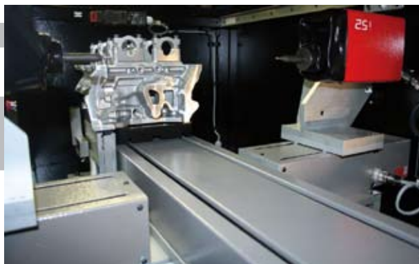
Engine block marking by two i52
