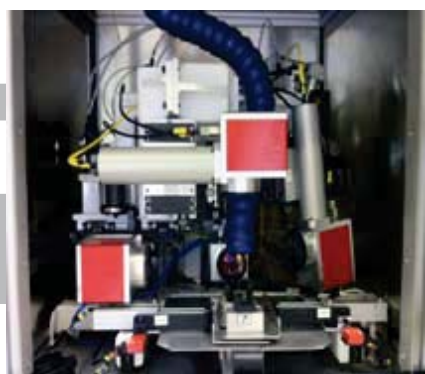
Four marks simultaneously on connecting rod by 4 galvano-heads
