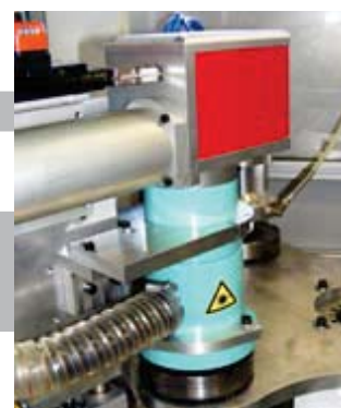
Laser tunnel protection
